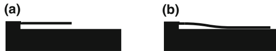
Fig. 13.5 a Micrometer sized cantilever beam. b If the beam is too long or too thin the minimum free energy state corresponds to the beam partly bound to the substrate. Surface roughness lowers the binding energy (per unit area) and hence stabilizes the non-bonded state in (a)
